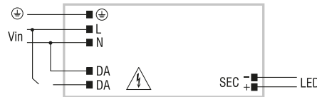
PUSH SWITCH diagram Collegamento PUSH SWITCH
